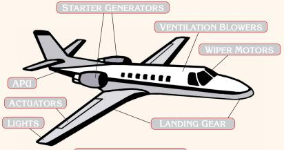
Landing Gear Starter Generators Wiper Motors Hydraulic Actuators Landing Gear Motors Oscillating Lights Fuel Shutoff Valves Blower Motors APU
